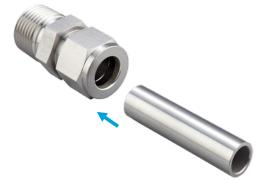
1. Insert well prepared tubing into VEE-LOK two ferrule tube fittings until tubing end is firmly seated on the body shoulder.
