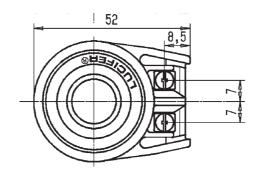
All dimensions are in mm Dimensional Drawing  $N^{\circ}$  11
