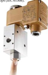
**Manual Reset function** These valves close when the electrical signal fails. When the electrical signal comes back, the valve remains closed, it has to be reset manually.
